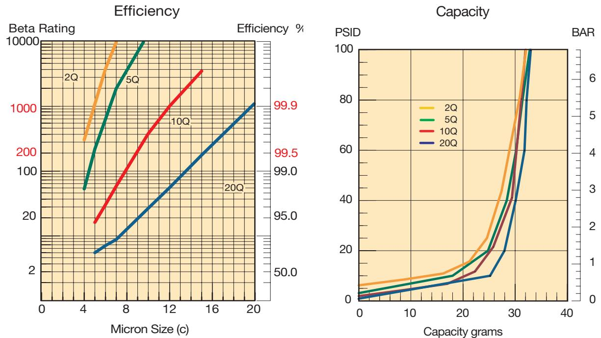
Results typical from Multi-pass tests run per test standard ISO 16889 @ 15 gpm to 100 psid terminal - 10 mg/L BUGL
