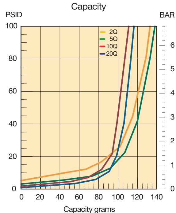
Results typical from Multi-pass tests run per test standard ISO 16889 @ 70 gpm to 100 psid terminal - 10 mg/L BUGL
