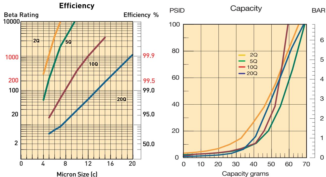
Results typical from Multi-pass tests run per test standard ISO 16889 @ 30 gpm to 100 psid terminal - 10 mg/L BUGL
