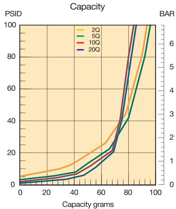
Results typical from Multi-pass tests run per test standard ISO 16889 @ 45 gpm to 100 psid terminal - 10 mg/L BUGL
