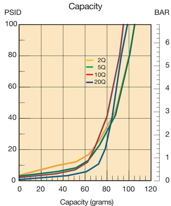
Results typical from Multi-pass tests run per test standard ISO 16889 @ 45 gpm to 100 psid terminal - 10 mg/L BUGL
